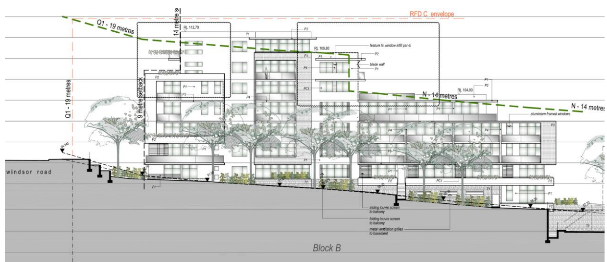
ELEVATION DIAGRAM SHOWING BLOCK B EXCEEDING THE HEIGHT LIMITS IN Q1 & N ZONES
